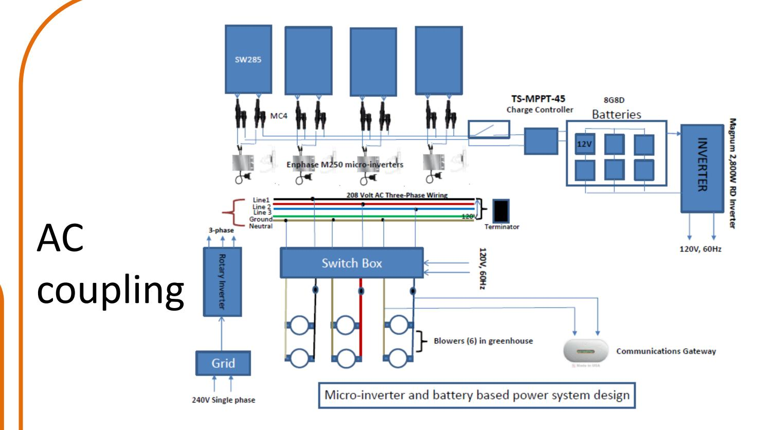
Hybrid Micro-inverter Battery-Based Power System
