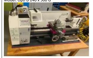
A lathe is a machine that rotates a workpiece on a spindle to cut away excess material, using cutting tools and drill bits with different diameters that are applied to the workpiece to produce a symmetrical object. This particular lathe is a manual operated Lathe.
