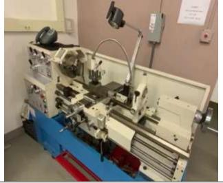
A lathe is a machine that rotates a workpiece on a spindle to cut away excess material, using cutting tools and drill bits with different diameters that are applied to the workpiece to produce a symmetrical object. This particular lathe is a manual operated Lathe.
