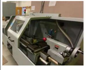
A lathe is a machine that rotates a workpiece on a spindle to cut away excess material, using cutting tools and drill bits with different diameters that are applied to the workpiece to produce a symmetrical object. (CNC) Computer Numerical Control Lathe Machines are capable of producing a variety of shapes, cuts, and details on a rotating work part. CNC lathe machine could be programmed to make difficult cuts on tough materials and produce quality pieces at a high rate.
