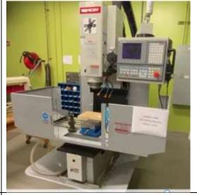
CNC Milling Machine allow intricate designs to be crafted from a full range of materials, steel, ceramics, plastic compounds, wood, composites, etc. (CNC) computer numerical control milling is a machining process which employs computerized controls and rotating multi-point cutting tools to progressively remove material from the workpiece and produce a custom-designed part or product.
