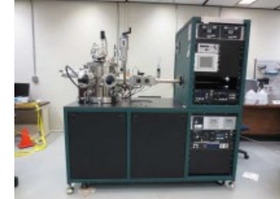
AJA International Sputtering machine 2DC powered and 3 RF powered guns. Along with plasma oxidation capabilities
